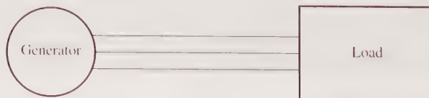
Figure 5–22 | A single generator supplying a load.
