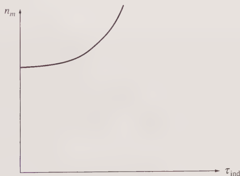
Figure 8–46 | The torque–speed characteristic of a differentially compounded DC motor.
